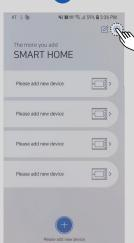
Press Add new device. Then, it'll require PIN number and you can find from the videophone. Then, installation complete.
